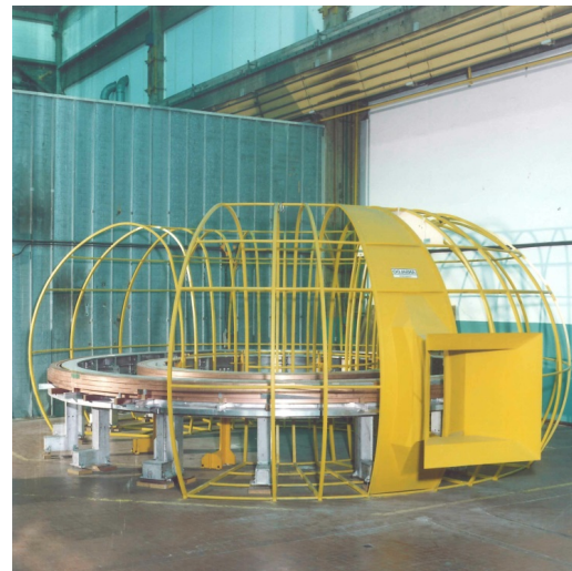
1:1 scale dummy coil to assess the feasibility of the coil inside the vessel
